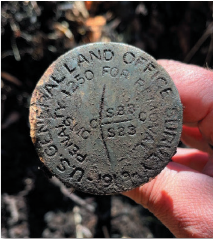
An original GLO brass cap from 1919 Resurvey found disturbed. Note the markings for the many Meander Corners encountered.
