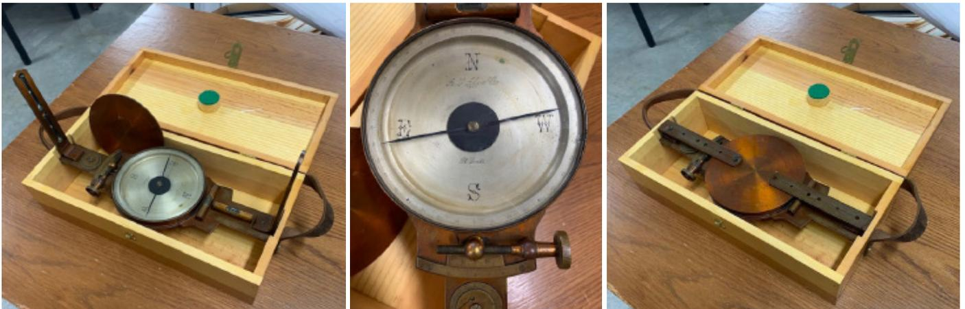
***This compass is marked "A.S. Aloe & Co. 7567, St. Louis". It has folding sights (an unusual feature) and an outkeeper. The serial number records for Aloe are not extant, so the date of manufacture for this compass is unknown. The instrument is from the collection of Dick Elgin. The custom box was built by his late father, Bob Elgin.***
