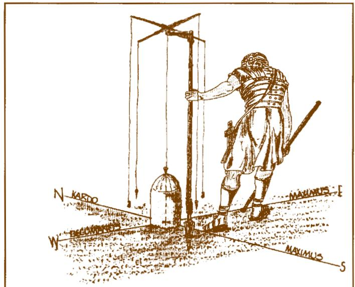
Figure 4. Army surveyor or *gromaticus* with *groma* at initial point of a survey. Drawing from M. J. Ferrar, *Cartography Unchained* website. Used with permission.
