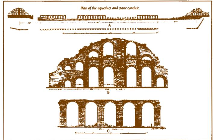
Figure 13. Towers and venter bridges for the Aspendos aqueduct. Drawing from Lanckoronksi, 1890.
