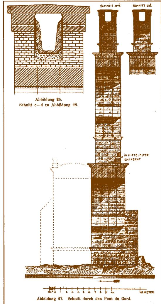
Figure 11. 1910 end section drawings by Stubinger.
