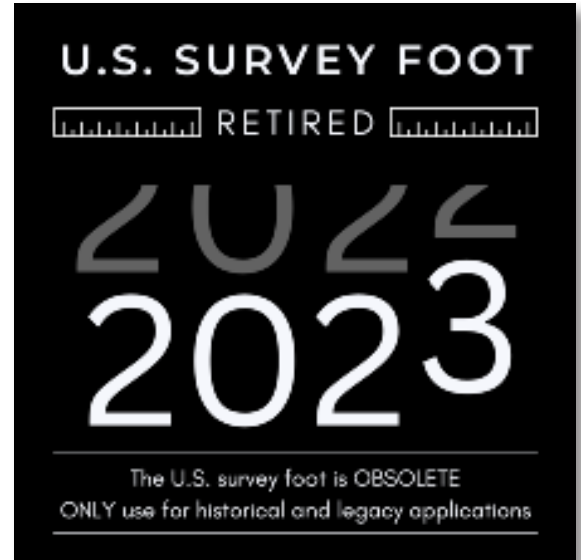
The U.S. survey foot is obsolete. Only use for historical and legacy applications. Credit: NIST
