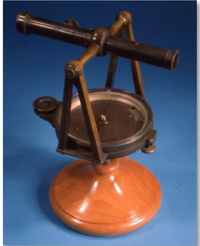
(left) Solar Transit by W. & L.E. Gurley; Troy, NY. (right) This is one of the first transits made in American. William J. Young, Philadelphia. Three minute least count, bullseye bubble. Was made in the very early 1830s.
