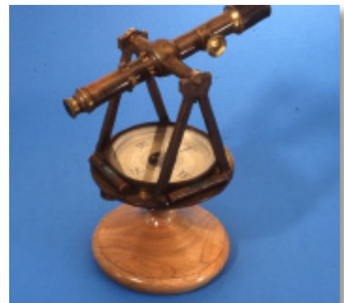
Telescopic compass (not a transit) by Blattner & Adam; St. Louis, MO. Late 1800s
