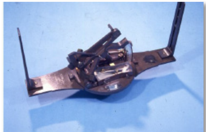
(left) The standard American vernier compass by W. & L.E. Gurley. This form with vernier, outkeeper, sights, level vials, was made from about 1860 and remained in the Gurley catalogs into the 1930s. It attached to either a tripod or Jacobs Staff. (right) A rare Solar Compass by a very rare maker, John S. Hougham; Franklin, IN. Compass was made about 1861.
