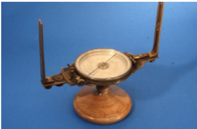
(left) The standard American vernier compass by W. & L.E. Gurley. This form with vernier, outkeeper, sights, level vials, was made from about 1860 and remained in the Gurley catalogs into the 1930s. It attached to either a tripod or Jacobs Staff. (right) A rare Solar Compass by a very rare maker, John S. Hougham; Franklin, IN. Compass was made about 1861.
