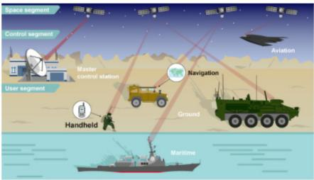
The Global Positioning System Involves Satellites, a Ground Control System, and Receivers
