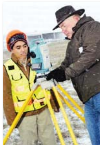
Philip Adams teaches a student how to set up a total station.
